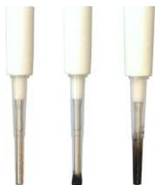
Left: extended magnet and tip without any particles. Middle: particles collected only on the apex of the tip. Right: a larger amount of particles collected using the full power of the magnet.
